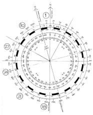
invented the pro- FIGURE 3. "32" POINT MAGNETIC COMPASS. portional compass.
